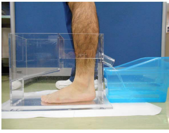
Figure 2. Measurement of Foot and Ankle. Measurement of Foot and Ankle by Water-Filled Volumetric Edema Gauge.
